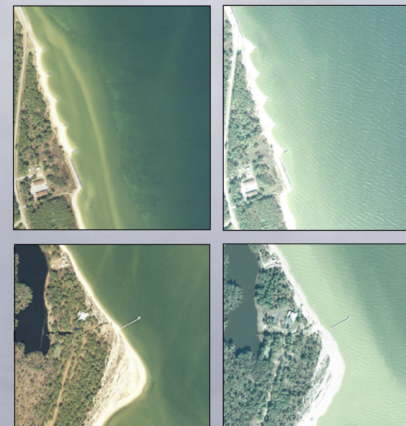
Pre- and post-storm photos showing the disruption of nearshore bars and the effectiveness of sand-trapping groins (above) and the reconfiguration of Point No Point, an incipient cusate foreland (below). Chesapeake Bay, St. Mary's Co. [10]
