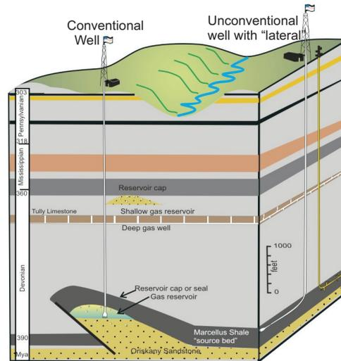
**Figure 4. Conventional versus unconventional gas well drilling. In unconventional drilling the source bed becomes the gas reservoir.**
