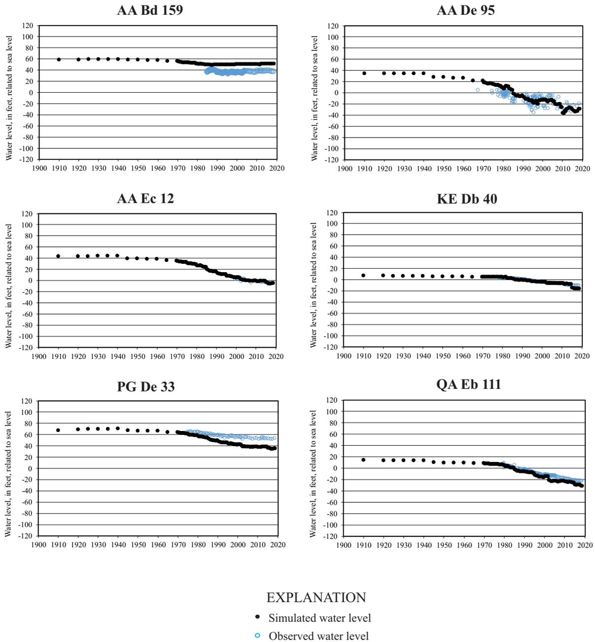
**Figure 5. Hydrographs of observed and simulated water levels in wells screened in the Upper Patapsco aquifer system, 1900-2018.**
