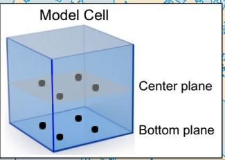
**Figure 18b. Particle paths in the Upper Patapsco aquifer system at simulated maximum withdrawals with a 2x2 array of particles placed on the bottom face of the model cell.**
