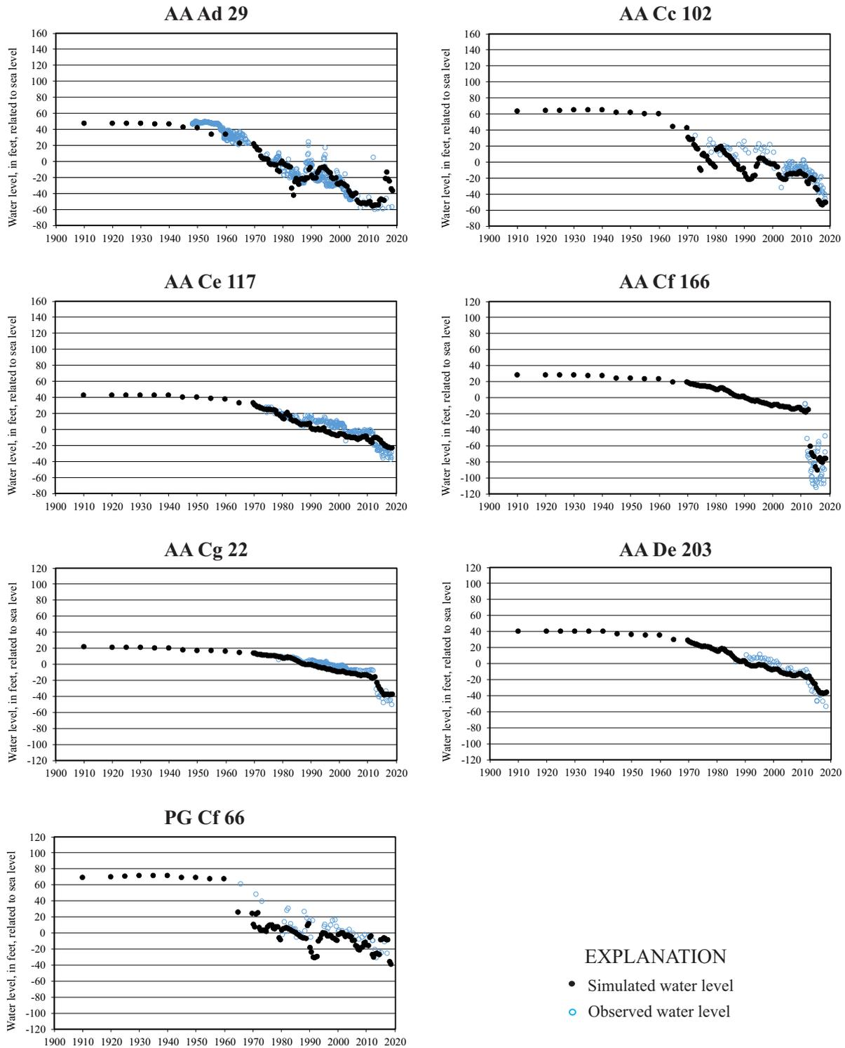
**Figure 7. Hydrographs of observed and simulated water levels in wells screened in the Patuxent aquifer system, 1900-2018.**
