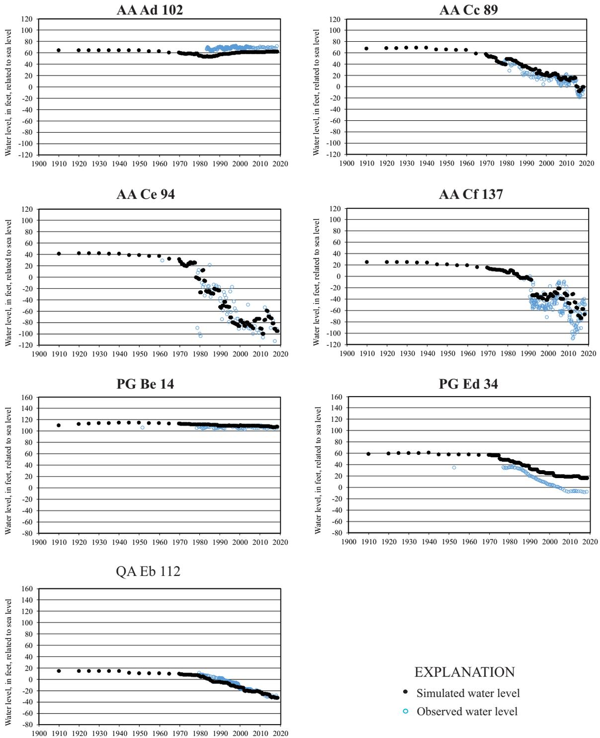
**Figure 6. Hydrographs of observed and simulated water levels in wells screened in the Lower Patapsco aquifer system, 1900-2018.**
