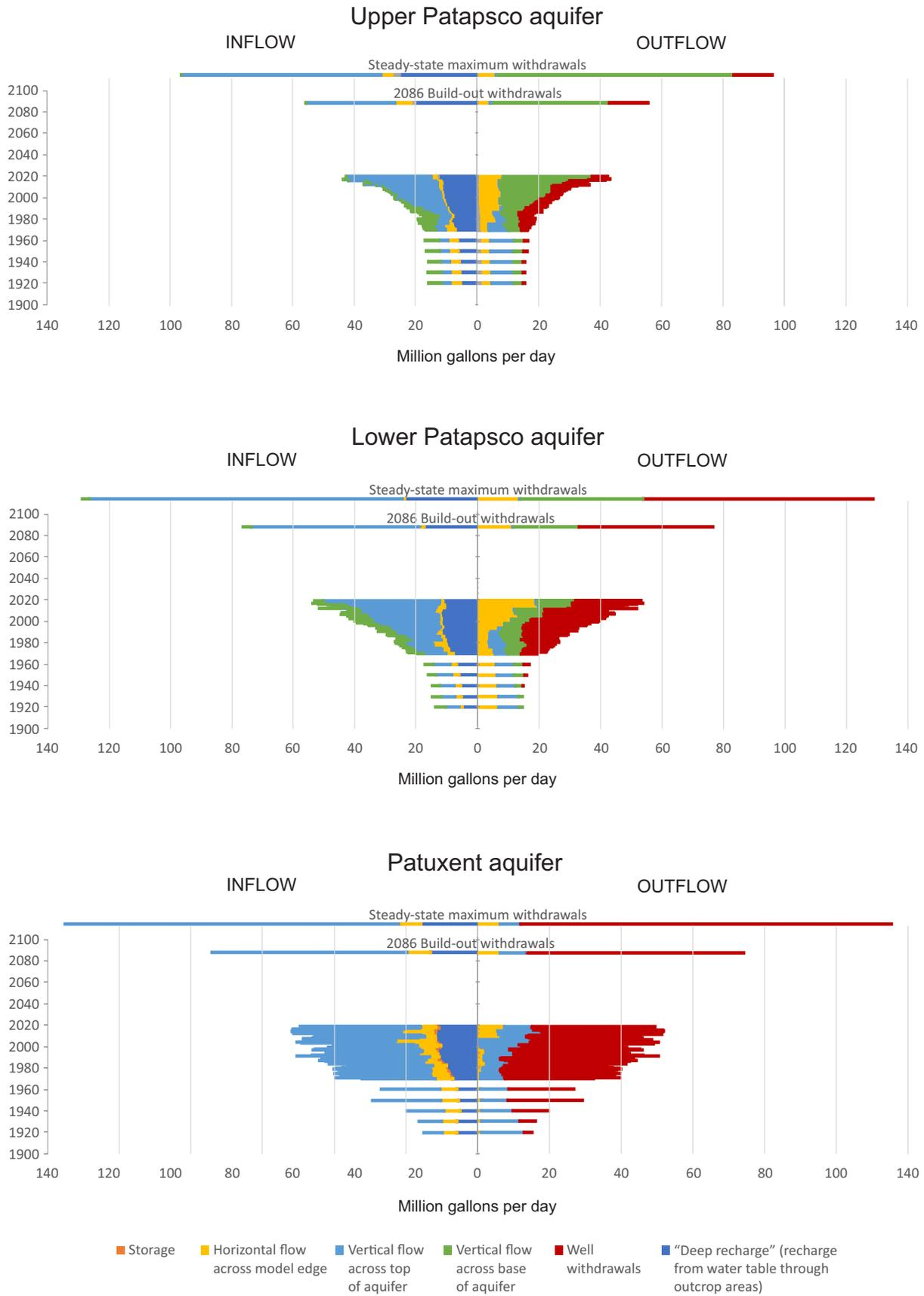
**Figure 15. Variations in simulated water budget over time in the Upper Patapsco, Lower Patapsco, and Patuxent aquifer systems.**
