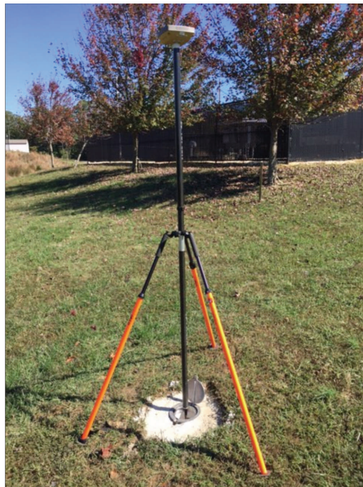
Figure 13. Photo showing GPS receiver.
